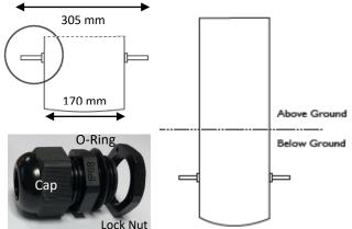
is on the outside of the tube, and secure in place with the locking nut inside the tube. Remove the domed cap, push the cable through the cap, threaded gland and then the locking nut. Secure the cap in place, screwing clockwise, when the desired length of cable has been pulled through to reach the bulb holder at the top of the tube with plenty of slack.
